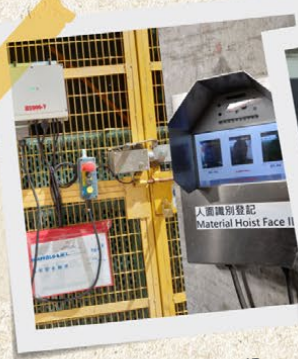
Safe Material Hoist with Face ID registration and electro-magnetic locking system
